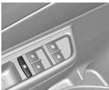
Pressione o interruptor
