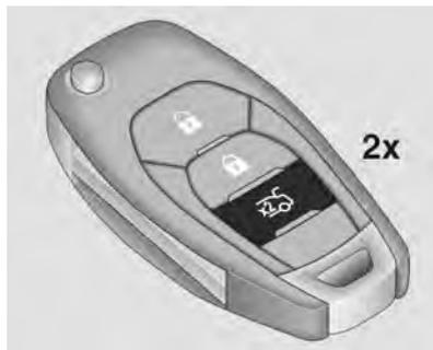
A tampa do porta-malas é destravada junto com as portas pressionando
