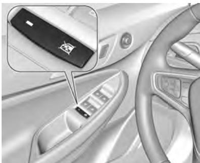
Pressione o interruptor
