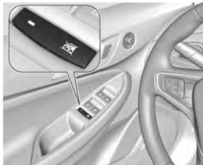
Pressione o interruptor
