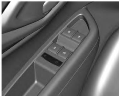
Pressione o interruptor
