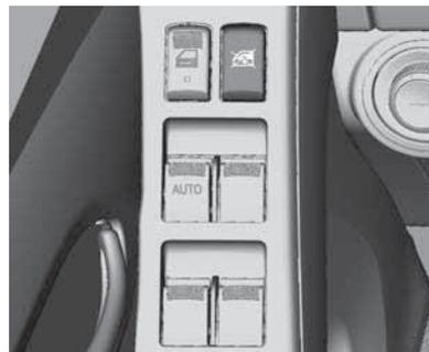
Pressione o interruptor
