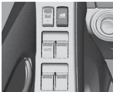
Pressione o interruptor
