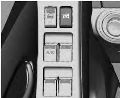
Pressione o interruptor
