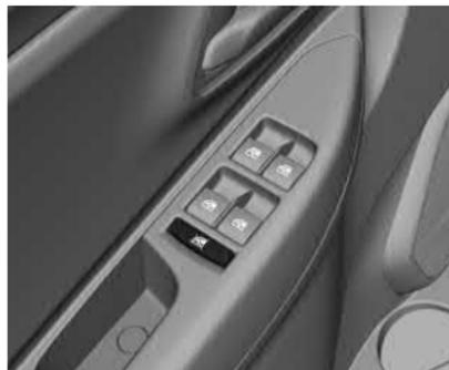
Pressione o interruptor
